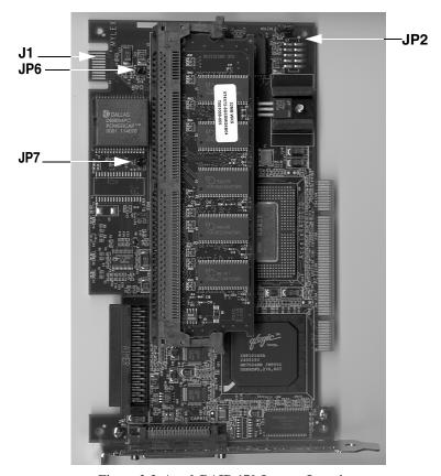
Figure 2-3. AcceleRAID 170 Jumper Locations
